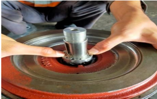
Gambar 4. 14 Proses Pemasangan Mechanical Seal (Sumber : PT. Wilmar Nabati Indonesia)
