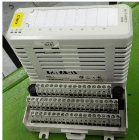
Gambar 3.9 System I/O S800
