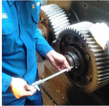
Gambar 4. 25 Pengambilan data drive NDE
