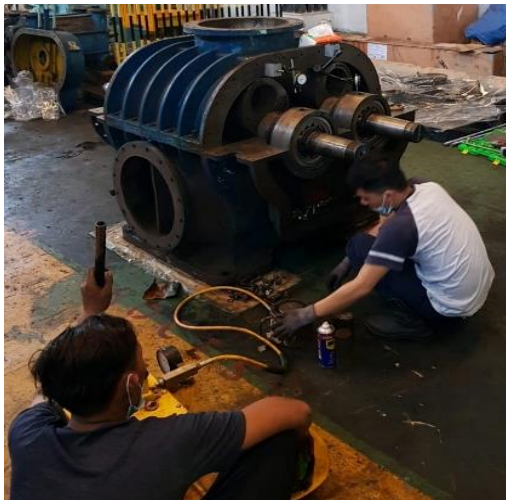
Gambar 4. 42 Setting radial clearance lobe to casing
