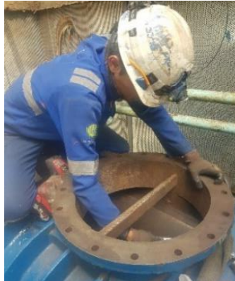
Gambar 4. 21 Pengukuran radial clearance lobe
