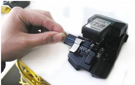
Gambar 4.2 Memotong Core
