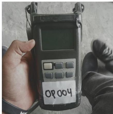
Gambar 3. 10 Optical Power Meter (OPM)
