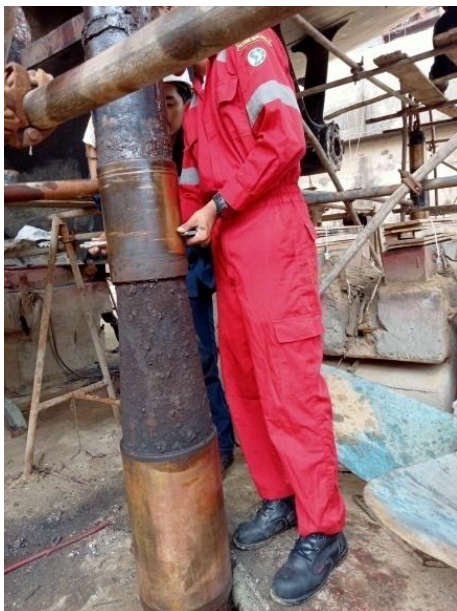
Gambar 2.21 pengukuran diameter shaft
