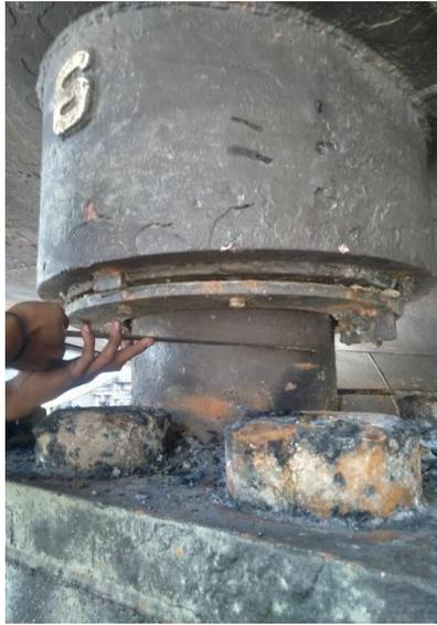
Gambar 2.11 mengukur diameter as daun kemudi
