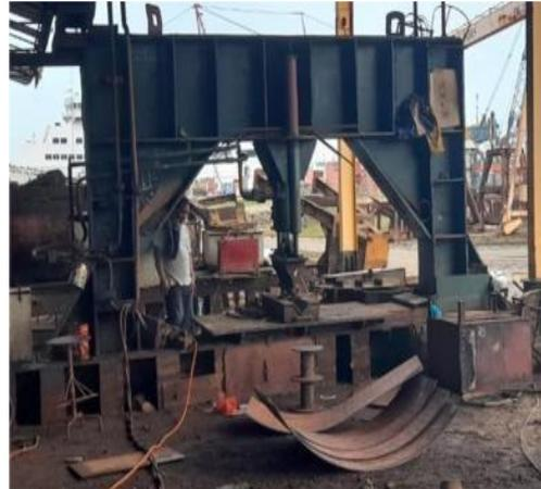
Gambar 1.13 Mesin Bending
