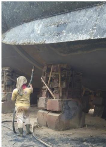
Gambar 2.1 proses sand blasting
