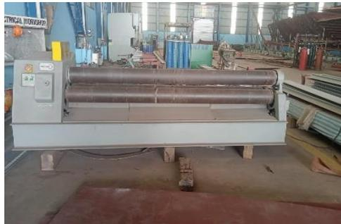
**Gambar 2.60** Mesin Bending
