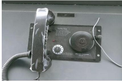
**Gambar 2.26** *Sound Power Telephone*
