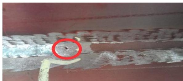
**Gambar 2.108** Cacat Las Lubang Pin
