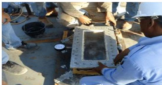
**Gambar 2.96** *Prosedur Vacuum Test*
