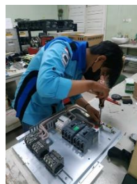
Gambar 2. 20 Merangkai Power Distributed Panel
