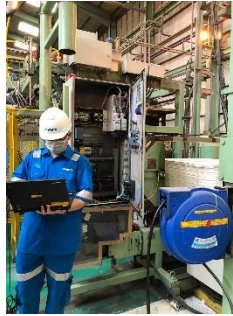
Gambar 2.15 Proses setting PLC diarea Pulp Dryer 3
