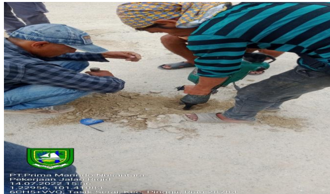
Gambar 4.10 Proses Pengujian Core Base
