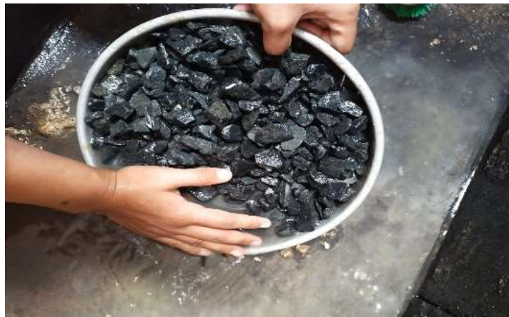
Gambar 3. 5 Pengujian kadar lumpur agregat kasar
