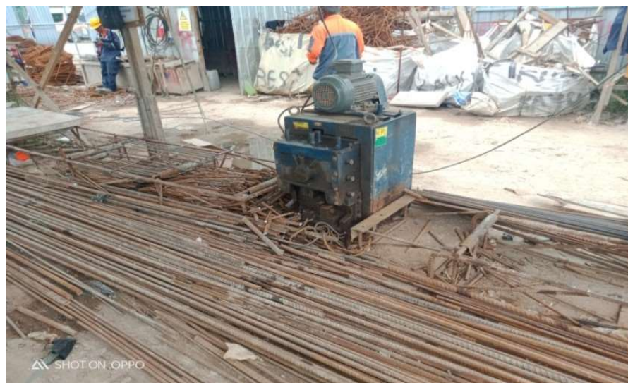
Gambar 2. 3 Mesin Bar Cutter
