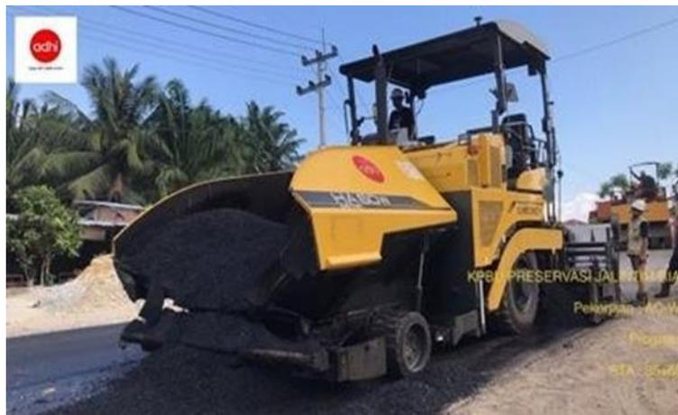
**Gambar 3. 2 Asphalt Finisher**
