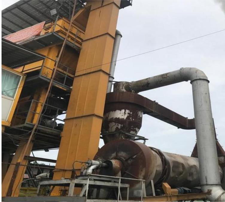
**Gambar 4. 13 Elevator Panas (Hot Elevator)**
