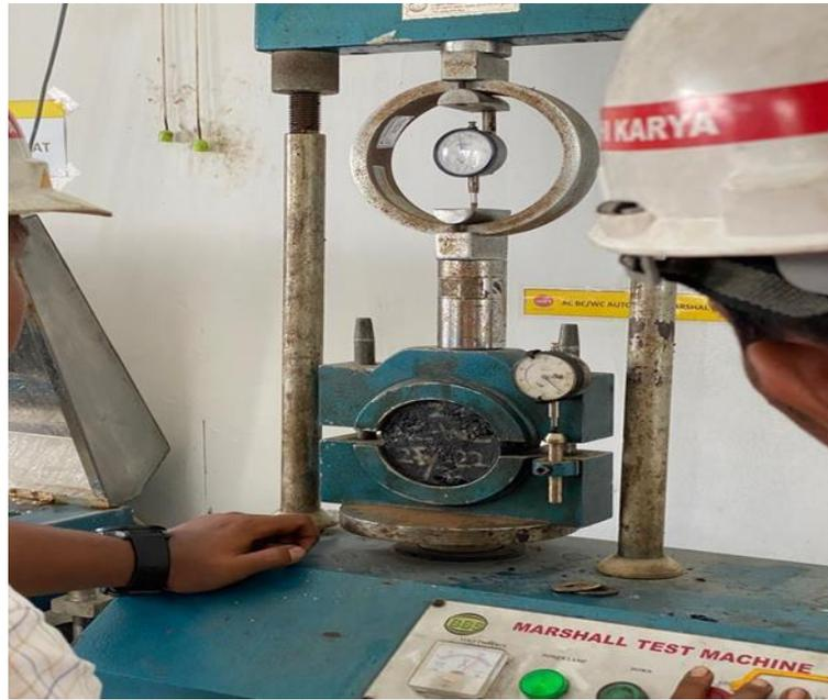
**Gambar 3. 19 Pengujian Marshal Test**
