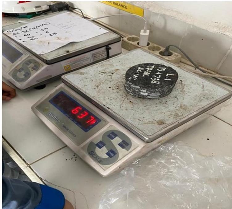
**Gambar 3. 18 Penimbangan Hasil Coredrill**
