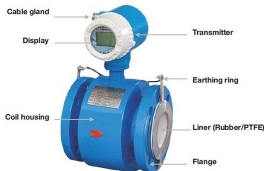
Gambar 3. 27 Bagian-bagian flow meter
