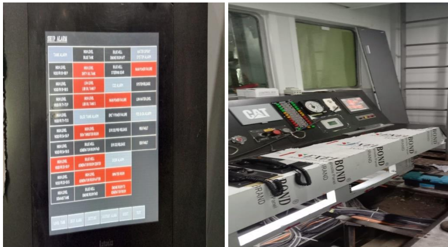
Gambar 2.36 pengujian ship alarm (Fuel Tank and Ship Alarm Monitoring) KP.WISANGGENI 4. Hari Kamis (Tanggal 24 November 2022)
