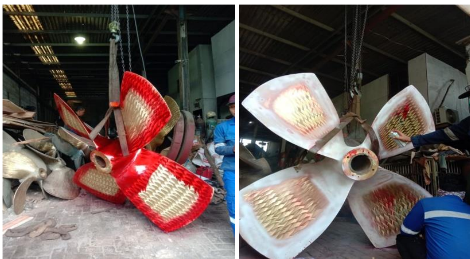
Gambar 2.39 Proses Non-Destructive Test Propeller TB.TINJU
