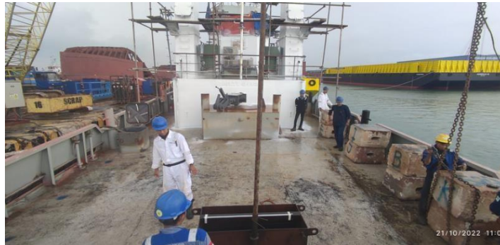
Gambar 2. 38 Proses Inclining Test
