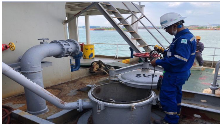
Gambar 2.30 Free Gas Survey MT.Sc Commander L VII
