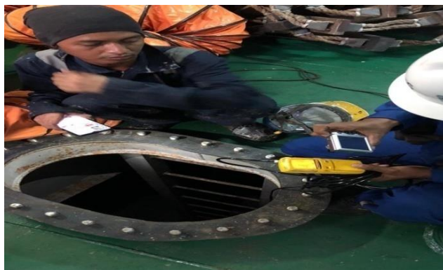
Gambar 2.29 Free Gas Survey MV. Pelita
