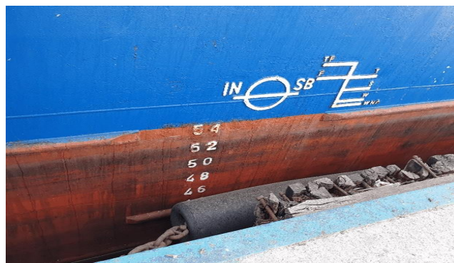
Gambar 2.26 Draft Survey MV. Surya Pertiwi Surabaya
