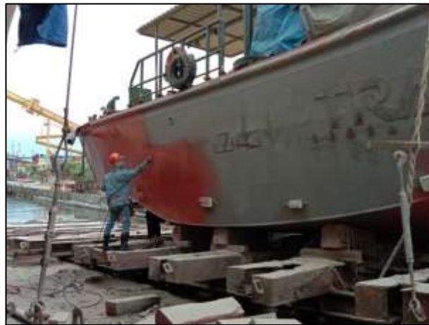
Gambar 2.67 Proses pengecatan anti corrosive
