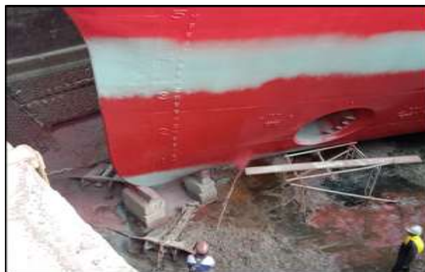
Gambar 2.20 Proses pengecatan Anti Fouling
