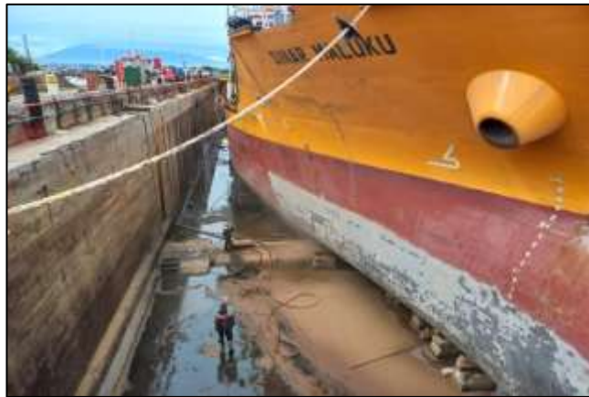
Gambar 2.81 Proses sand blasting kapal Sinar Maluku
