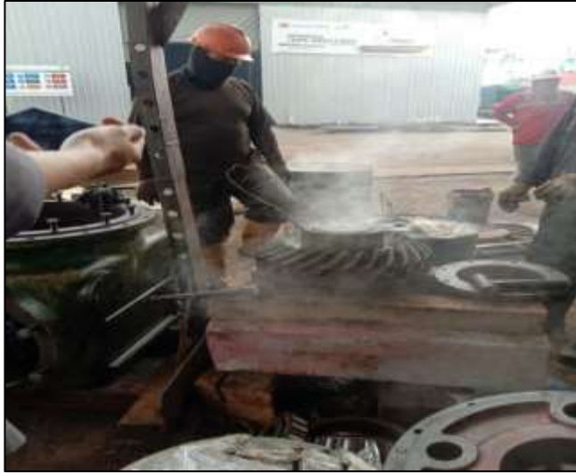
Gambar 2.29 Proses pemasangan bearing upgear
