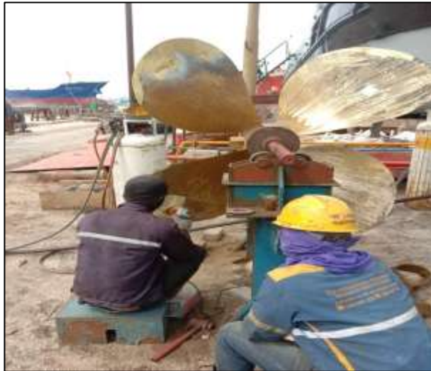
Gambar 2.21 Proses repair propeller kapal
