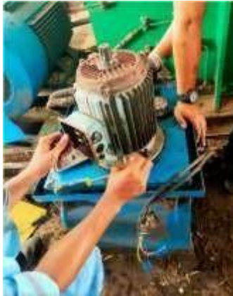
Gambar 2.7 Photo open install motor 3 phasa (Suber:dokumentasi 2022)
