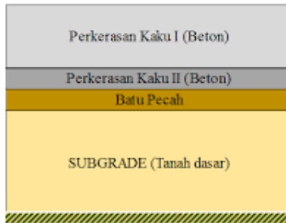
Gambar 3.2 Perkerasan Kaku (Sumber: https://www.sisipil.com/perkerasan-kaku/ )
