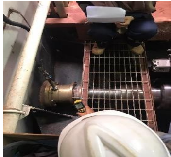
Gambar 3.2 Pencatatan Temperatur Cooling Engine dan Sistem Poros Kapal ( Bearing Gearbox, Gland Packing, Shaft, dan Stern Tube )
