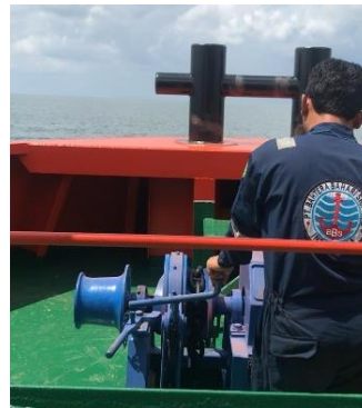
Gambar 3.9 Proses Saat Hoisting Anchor
