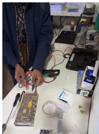
Gambar 3.6 Pengecekan Power Supply
