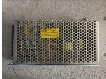
Gambar 3.15 Power Supply Sumber : PT.Mobilkom Telekomindo
