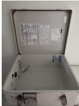
Gambar 3.12 Box RTU kosong Sumber : PT.Mobilkom Telekomindo
