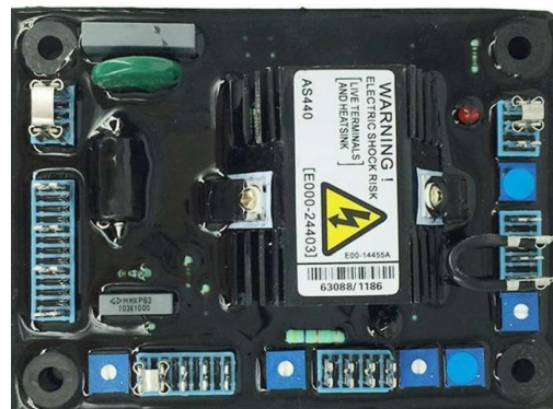
Gambar 3.1 Automatic Voltage Regulator (Sumber: http://anekacipta-eng.com/avr-pada-generator )
