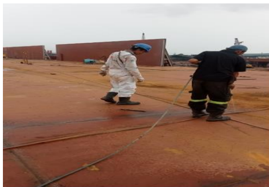
Gambar 2.73 Air Test External Diarea Main Deck
