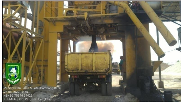
gambar 3.22 pengisian campuran hotmix kedalam dump truck
