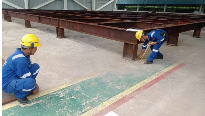
Gambar 2.20 Proses pengukuran layout PT.KSS
