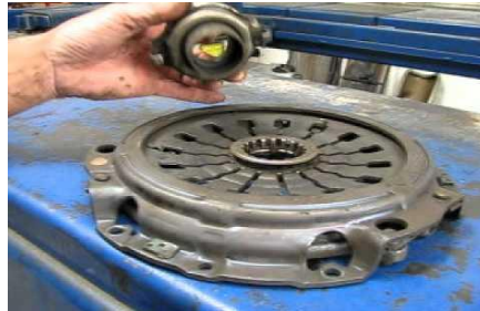
Gambar 4.5.3 Pengujian release bearing
