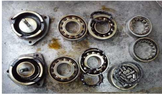
Gambar 4. 4 Kerusakan Bearing Pompa Condensat
