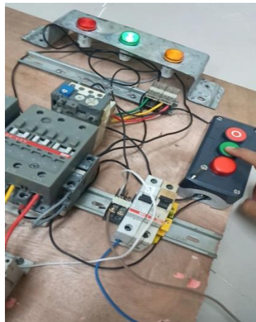
Gambar 2.7 : Merangkai Wearing DOL.
