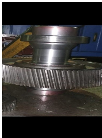
Gambar 4.5 Hollow Shaft Gear Sumber: PT. Indah Kiat Pulp&Paper
