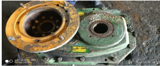
Gambar 4.2 Gearbox Compact Shredder Screw Sumber: PT. Indah Kiat Pulp&Paper
