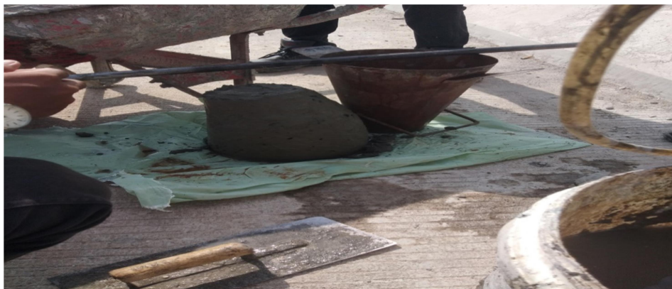
Gambar 3.17. Uji slump beton
