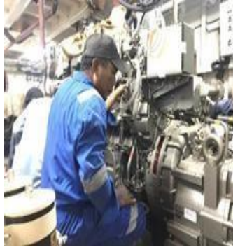
Gambar 3. 7 Proses Pengukuran Crank Shaft Deflection
