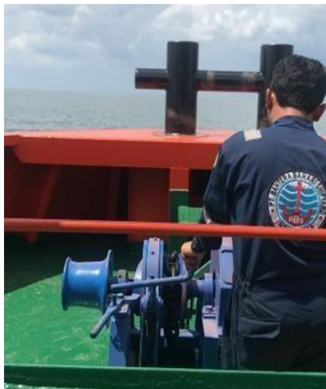
Gambar 2. 22 Proses Saat Hoisting Anchor
