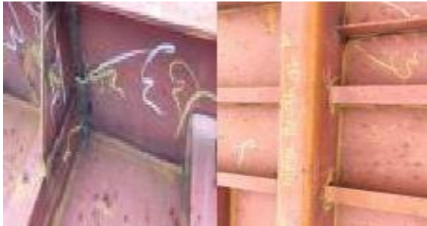
Gambar 2. 69 Visual Welding H-613
