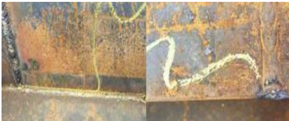
Gambar 2. 102 Visual Welding cacat star stop, undercat
