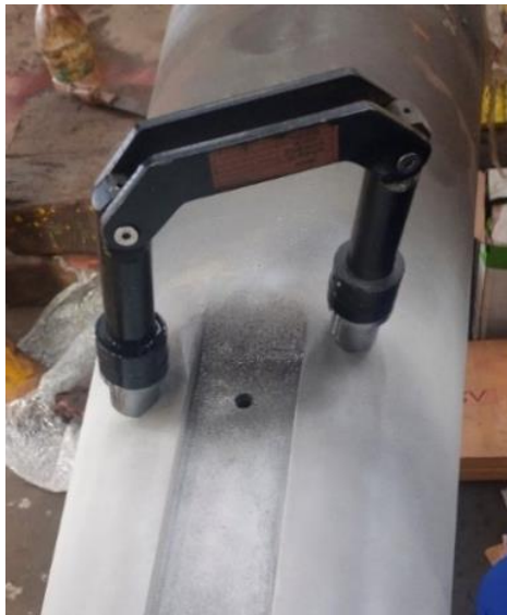
Gambar 2. 7 magnetic particle test bagian foreward
