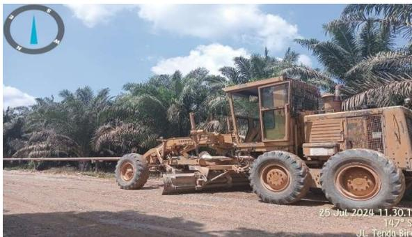
Gambar 3.5.Motor Grader
