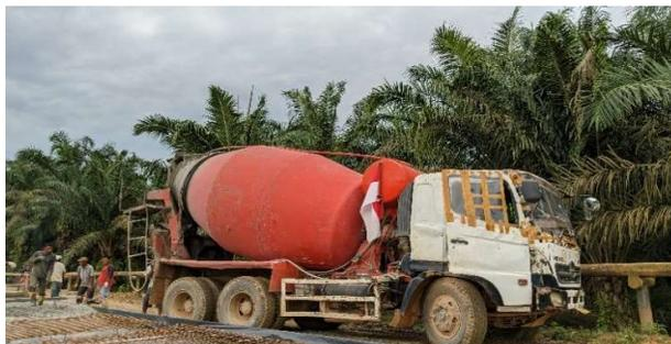
*Gambar 3 10. Concrete Truck Mixer*
