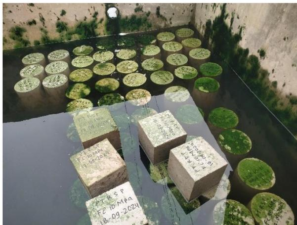
Gambar 3. 25 Sampel Pegujian Kuat tekan Beton
