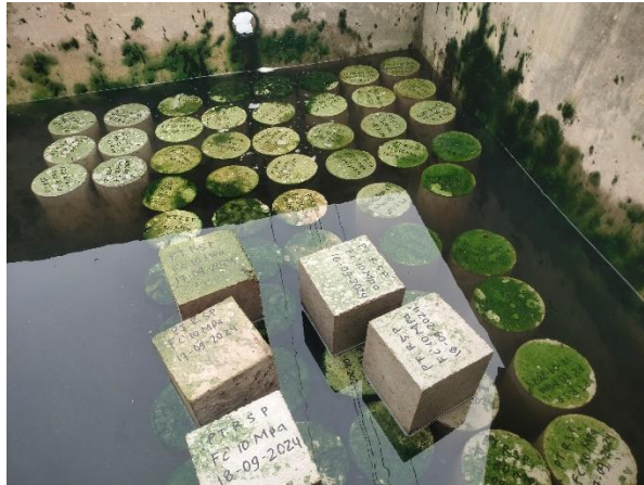
Gambar 3. 25 Sampel Pegujian Kuat tekan Beton
