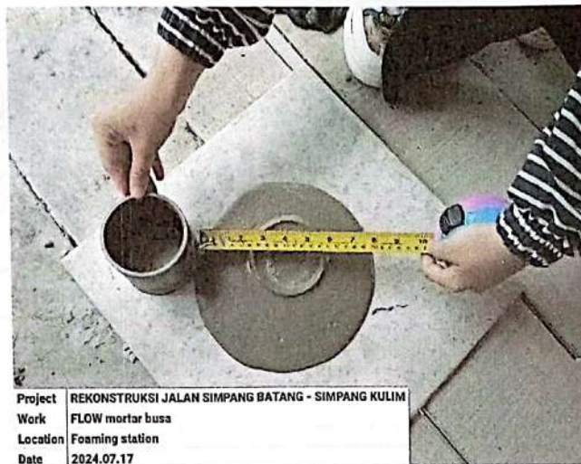
Project REKONSTRUKSI JALAN SIMPANG BATANG - SIMPANG KULIM Work FLOW mortar busa Location Foaming station Date 2024.07.17
