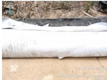
**Gambar 4. 1** Geotextile non-woven
