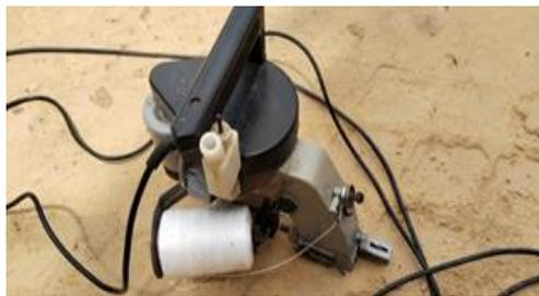
**Gambar 4. 3** Mesin Jahit Geotextile
