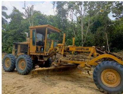
**Gambar 3.3** Motor Grader
