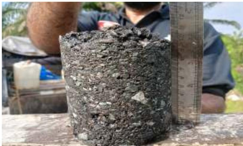
*gambar 4. 18 Hasil Core Drill*
