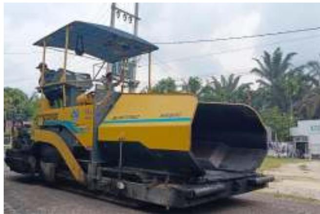
*gambar 4. 2 Asphalt Finisher
