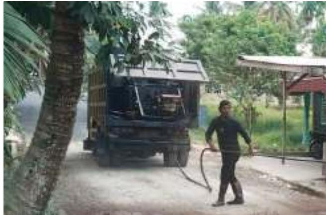
*gambar 4. 1 Asphalt Distributor*
