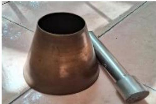
Gambar 3.19 kerucut abrams
