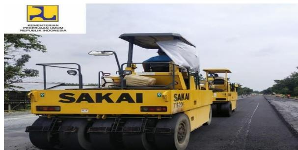
**Gambar 3. 9 Pneumatic Tire Roller (PTR)**
