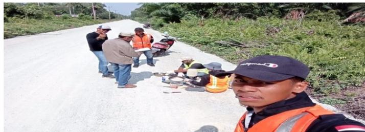
Gambar 3 23 Pengujian Sand Cone Base B
