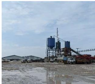
Gambar 2. 1 Mesin Batching Plant
