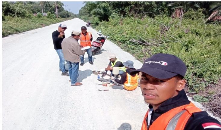
Gambar 1. 26 Pengujian *Sand Cone Base A (Density)*
