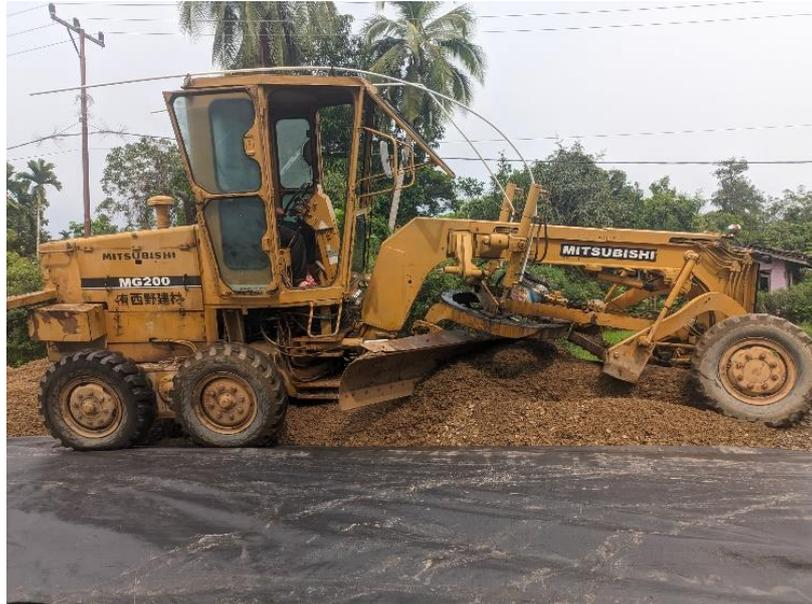
Gambar 3.6 Motor Grader
