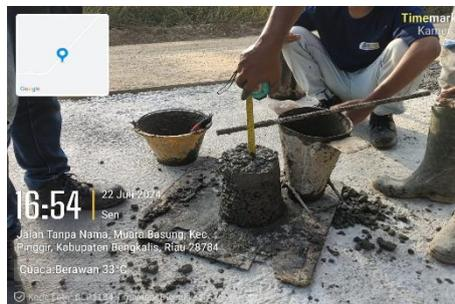
*Gambar 3. 14 Uji Slump LC
