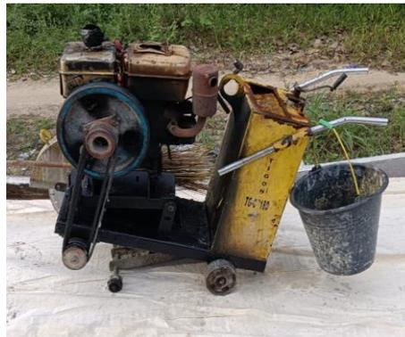
*Gambar 4. 10 Mesin Cutting Beton
