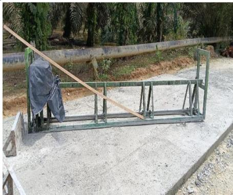
*Gambar 4. 4 Concrete Paver
