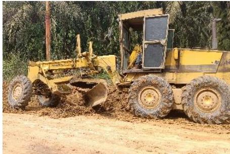
*Gambar 3. 1 Motor Grader
