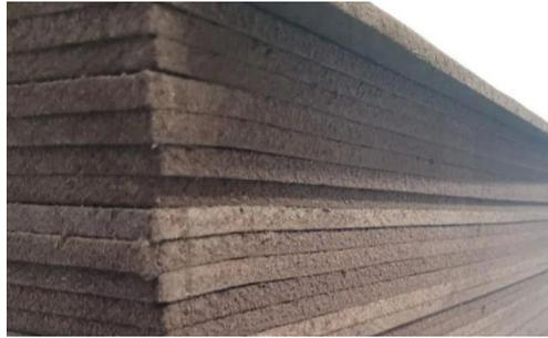
**Gambar 3. 18** *joint filler board*
