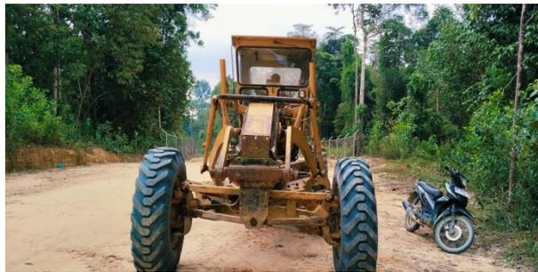
*Gambar 4. 1 (Alat Berat Motor Grader)
