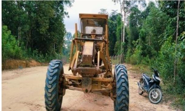
*Gambar 3. 3Motor Grader*
