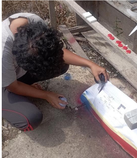
Gambar 4. 22 Proses Painting Hull (Sumber: Penulis)
