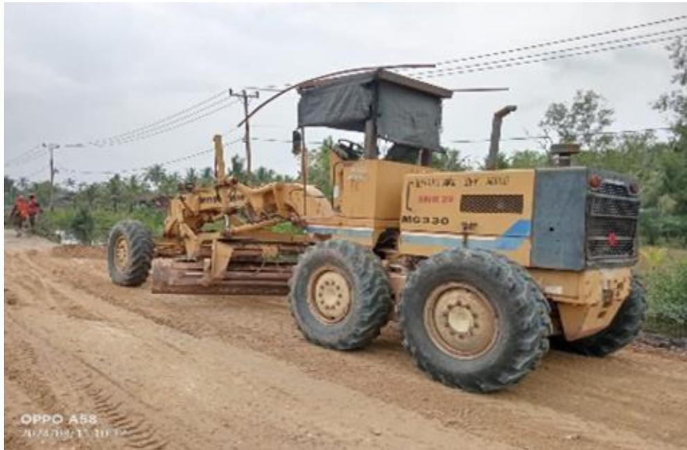
**Gambar 3. 2** Gambar Motor Grader
